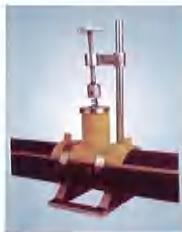
鞍型件焊接夹具 welding jig for saddle-shaped parts
